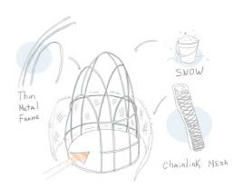
Each hut is individual and has its own height and diameter. They are also seasonal and easily erected. The base is a metal frame with a chain link mesh. There is pressed snow both outside and inside the buildings.
